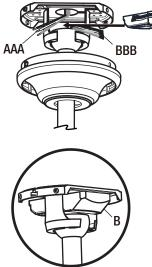
Receiver (B) correctly positioned in the mounting bracket.
