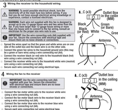
Turn the wire connecting nut (AA) upward and push the wiring
