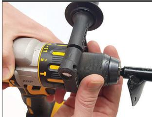
Check tightness regularly when digging to avoid stripping the head. With metal chucks, you can lock it by one click backwards after fully tightening.
