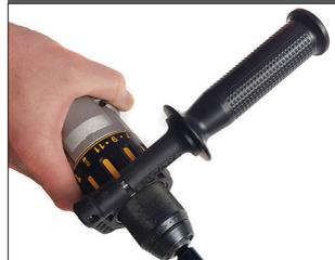
If you have a side handle for your drill it will make controlling the Power Planter easier. Hold drill firmly with two hands and have body in stable position.
