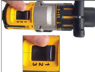
Do NOT operate on high speed. It is dangerous and ineffective to do so. Drill speed should be on Level 1 or Lo.
