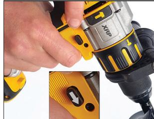
Ensure the drill is in Forward mode otherwise the Power Planter will just spin on the surface. It is marked with a forward arrow or the letter 'F'.
