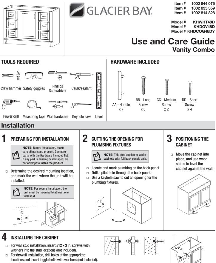
For concrete wall installation, drill 1/4 in. holes at the appropriate locations and insert #12 wall anchors, followed by #12 x 3 in. screws (not included).
