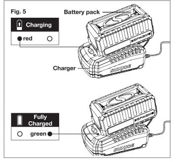
**4.** When the charger light turns green, the battery is fully charged (Fig. 5).
