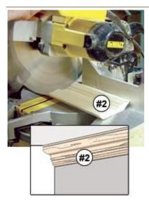
A coped joint is sometimes used when crown mouldings meet at inside corners. Coped joints help cover irregularities more effectively than mitred joints.
