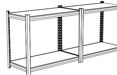
Shelving units can be assembled vertically or horizontally, as shown.
