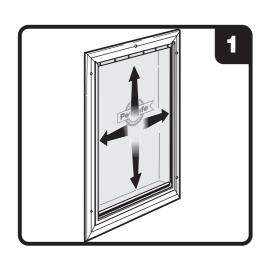
1. The flexible flap is adjustable to fit into frame correctly.
