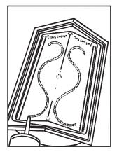
2. Apply a 1/8" bead of color match silicone sealant as illustrated.
