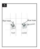
Connect the flexible hoses to the water supply valves (left to hot water and right to cold). Make sure flexible hoses are securely fastened before turning on valve.
