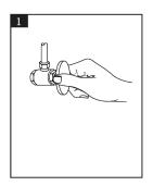
Clean all dirt and debris from supply valves before proceeding with installation. If you are replacing an existing faucet, remove the faucet from the sink and clean the surface thoroughly.
