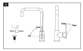
Pull the handle rightward in horizontal to turn on the mixer ,leftward in horizontal to turn off. The water will be connected to the sprayer when press the button on it.
