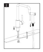
Drill a  $\varnothing$ 1-1/2"to $\varnothing$ 1-3/8"hole (2) and  $\varnothing$ 1"(3) in sink(1).Put the rubber washer through the bottom. Then install the faucet through the left hole on sink.
