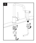
From underside sink, put on the plastic washer and metal washer in order and tighten with mounting nut by hand. Before final tightening, make sure spout and handle facing forward. Tighten the screws with tooling.
