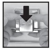
To lock in place, continue applying pressure on suction cup, then pull down square cap until it snaps closed.
