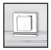
While applying pressure to suction cup, with the square cap in upward position, attach the wire product into the groove on the front of suction cup.
