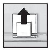
To remove, push cap upward to release suction cup back into flat position.
