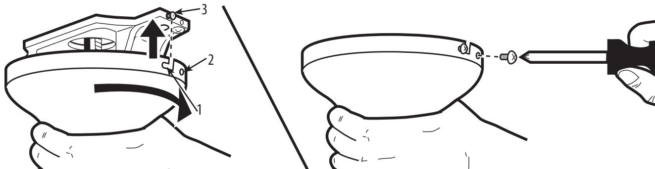
The canopy has two mating slots (1) and two mating holes (2). Position both slots on canopy directly under and in line with two screws in the mounting bracket (3). Lift the canopy, allowing the two screws to slide into the mating slots. Rotate the canopy until both screws from the mounting bracket drop into the slot recesses. Tighten screws securely. Install two screws into the mating holes of the canopy and tighten to secure the canopy to the mounting bracket.
