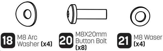
Attach the Step 23 to the Step 22 with four M8 Arc Washers **(18)** and four M8 Washers **(21)** and eight M8X20mm Button Bolts **(20)**.
