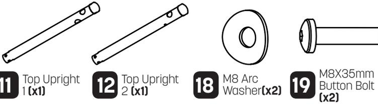
Fix the Top Upright 1 **(11)** and Top Upright 2 **(12)** with the M8X35mm Button Bolts **(19)**, M8 Arc Washers **(18)**.
