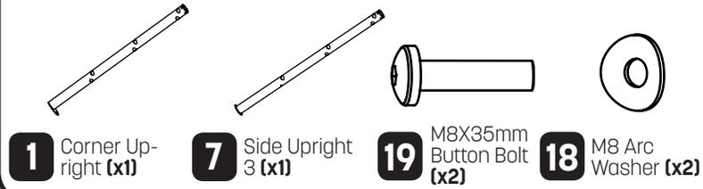
Fix the Corner Upright **(1)** and the Side Upright 3 **(7)** with two M8 Arc Washers **(18)** and two M8X35mm Button Bolts **(19)**.
