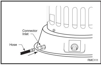
Fig. 6 Hose and connector inlet.
