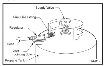
Fig. 5 Attach regulator with vent pointing down.
