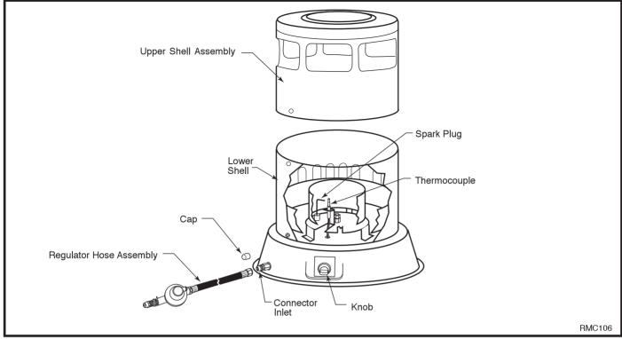
Fig. 1 Convection Heater parts identification.
