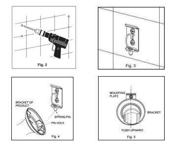
2. Take away the mounting plate after marking is done. Start to drill holes at the marked screw locations, Fig.2.
