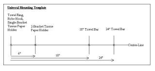
1. According to the different products you are going to install, check the corresponding mounting length needed as indicated on the Universal Mounting Template sheet.
