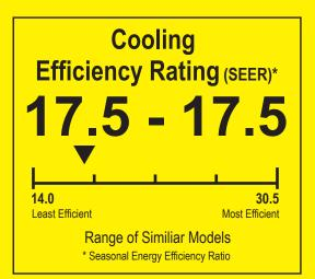
This system's efficiency ratings depend on the coil your contractor installs with this unit. The heating effiency rating will vary slightly in different geographic regions. Ask your contractor for details.
