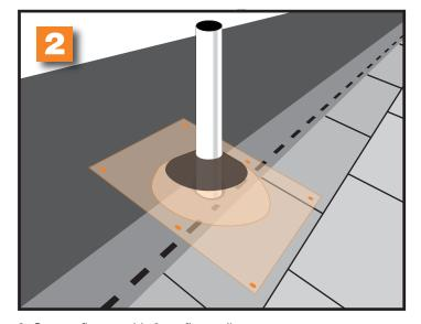
3. Secure flange with 6 roofing nails.
