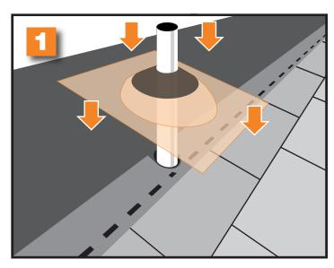
1. After shingling up to the pipe, slide flashing down over pipe.
