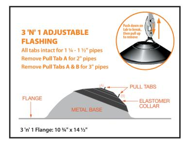
Using the pull tabs, adjust the size of the opening to fit the pipe.
