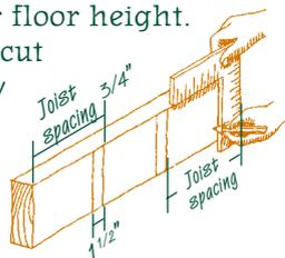
Nail the ledger board temporarily in place, the top flush with the chalk line. Since the ledger board will be supporting much of the deck's
