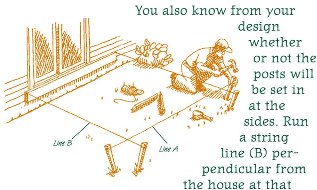
Example: for a 10' wide deck with 1' overhang on each side, you would start your line 4' out from the midpoint of the ledger board.
