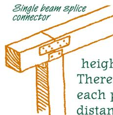
Since a single beam will lay on top of the posts, you will need to subtract the height of the beam from the posts. Therefore, make a second mark on each post below the first mark at a distance equal to the height of the beam. Then cut the posts at the second mark. Set the beam on top of the posts and attach with connectors and nails. Single beams are more susceptible to swaying, so use bracing wherever possible.
