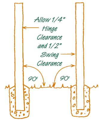
the first step comes when you are setting your face posts. Posts to either side of the gate should be absolutely plumb and set at least 24" in concrete.
