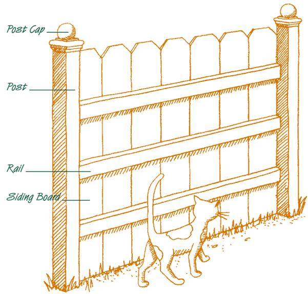
The components of most wooden fences include posts, rails, siding boards and post caps.
