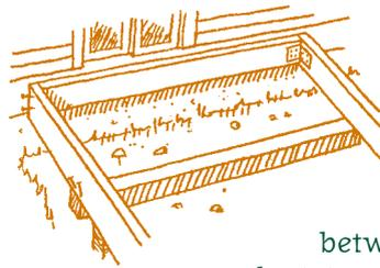
Nail into the edge of the ledger board, toenail into the top of the beam, then use an angle bracket to secure the connection between the ledger and the joist.
