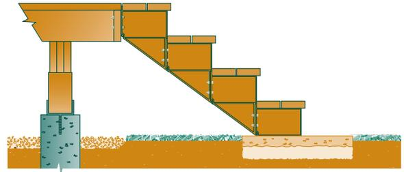
Stair Riser Brackets work in tandem to give strength and support while providing uniformity to your stair design. Easily bolted together, Stair Riser Brackets offer limited measuring to achieve maximum results.
