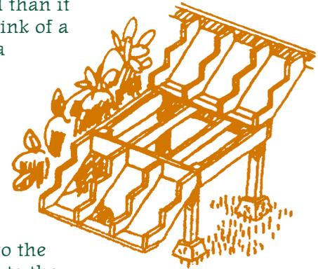
The most critical part of building stairs with a landing is the planning. You must first measure where you want the stairs to begin and end; then you can build the landing at the proper height, and in the proper position in relation to the deck.
