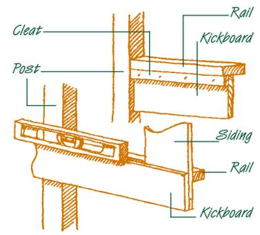
Apply gate hardware and facing boards to the frame with wood screws. When applying the siding boards to the gate, begin on the hinge side and cut the last board flush.
