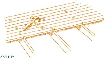
Secure the decking boards at each place where they cross a joist, using two nails or screws for 2x4's and three nails or screws for 2x6's. When using boards shorter than the deck length, make sure all board ends rest on a joist, and use different board lengths in order to stagger the splices.
