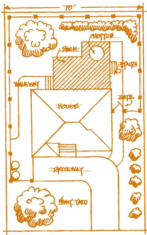
A 6- or 8-foot post spacing is most economical. Shorter sections that are needed to make the fence come out even should be placed at the corners or near the gates and buildings.
