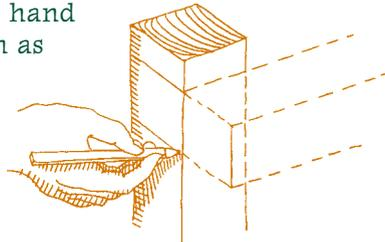
Once the beam is installed, use a framing square to mark where the interior joists will sit on the top of the beam.
