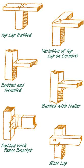
Rails are most easily set with galvanized metal\* fence brackets and nails. They may also be butted and toenailed, lapped, blocked or set with a dado. In each case, be sure to use galvanized\* nails. Drill pilot holes and stagger the nails in your rails to avoid splitting along grain lines. Attach the fence boards according to the style you have selected. Using a
