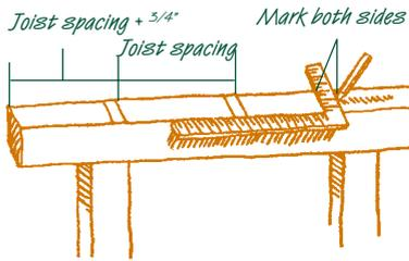
boards which "sandwich" the posts. Place the top of the beam boards flush with the mark and nail temporarily.
