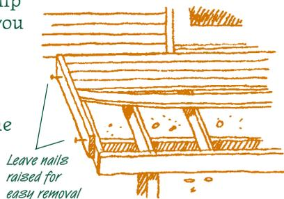
space the boards slightly for drainage (no more than 1/16" for wet decking, 1/8" for dry). As you proceed across your deck, measure the distance remaining and alter your spacing in order to avoid a large gap at the end.
