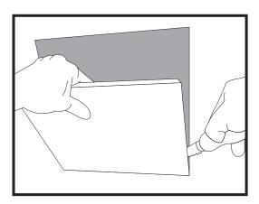
2) Cut along the lines that were traced from step 1. Use a keyhole, hand or jig saw to make the cut into the wallboard. Once the wallboard is cut, remove the loose center section.
