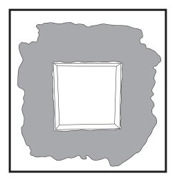
7. Apply a skim coat of Polymer Modified Thinset over the mesh tape to secure the joint between PolyNiche, and the wallboard. Flash out thinset if nessecary. Once the thinset is cured, a coat of waterproof membrane may be rolled or brush on.
