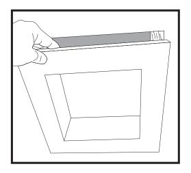
**4.** Place PolyNiche into the wall with the opening side facing out. Gently push PolyNiche into position until the frame of PolyNiche sits flat against the vertical wood supports. PolyNiche should now be flush with the ½" wallboard.
