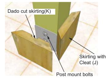
**24.** Locate all Post Skirting pieces. Position 2 post skirtings around the base of post as shown above. Use 1 Post Skirting with Cleat - 1 1/2" x 9" x 7 1/4" (Part J) and a Post Skirting with Dado Cut - 1 1/2" x 9" x 7 1/4" (Part K) initially. Cleat piece should be aligned opposite post mount hardware and dado piece aligned with post mount bolts (hardware).
