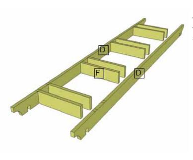
**12.** On a flat surface, position Ladder Blocking (F) where marked on top edge of Joist (D) and screw with 2 - 2 1/2" screws per end. Ladder Blocking should be flush with top and bottom of Joist with all notches facing down.
