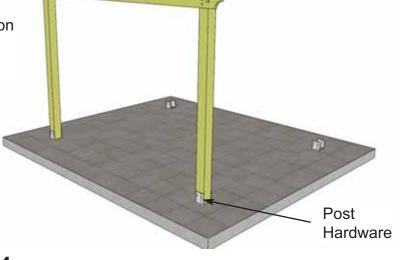
**4.** Secure Post to Post Hardware with appropriate hardware such as lag bolts or a sufficient number of screws.(Hardware Not Supplied)
