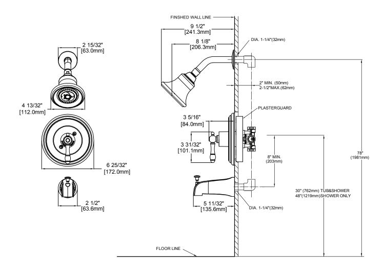
Showerhead max. flow rate: 2.5 gpm (9.5 Lpm) at 80 PSI Tub spout min. flow rate: 2.4 gpm (9.1 Lpm) at 20 PSI
