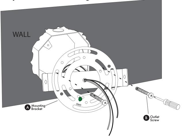
Align mounting bracket (A) with outlet box and secure with outlet screws (B).
