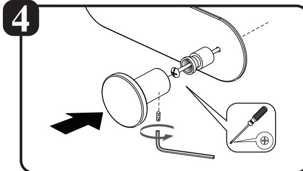
Place backplate against the wall, secure mounting pins with the screws, tighten set screws.
