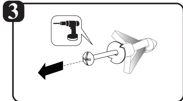
Use an electrical screwdriver to tighten the screws. This will collapse the molly bolts tightly to the wall. Unscrew the screws from the molly bolts.
