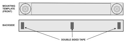
Use a level when sticking the template to the wall. Mark the wall through the template to spot the drill holes for the first 2 brackets. For the third bracket, you will be shifting the template horizontally left or right depending on your prefences. When ready, mark the final holes.
