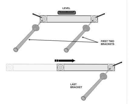
Remove the template and drill holes at the marked locations. Firmly seat drywall anchors using a malet and use screws to mount the brackets.
