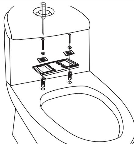
Loosely install the mounting plate with the plastic anchors, washers, and guides provided.
