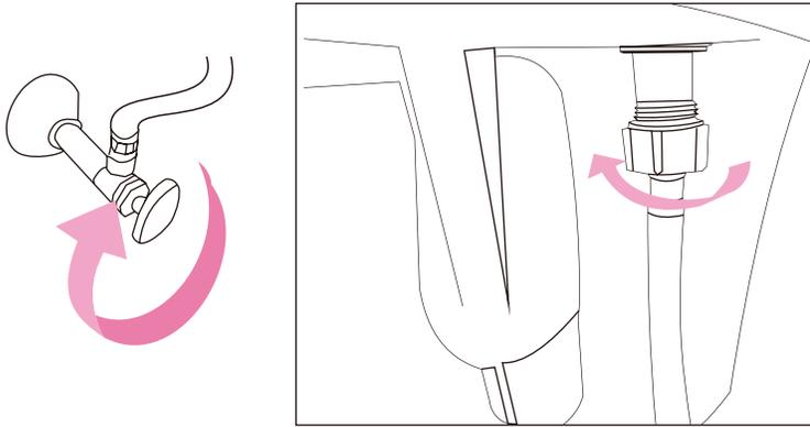
Turn off the inlet valve, and unscrew the supply hose from the toilet.
