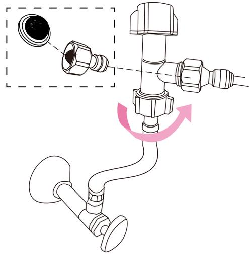
Screw the water supply hose to the Tee joint. Note that the filter is located in the reducer.
