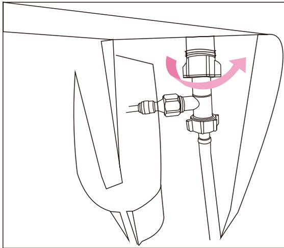
Screw the Tee joint to the toilet water inlet coupling.
