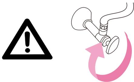
1. Turn off the water inlet valve before starting the installation of the smart toilet seat.
