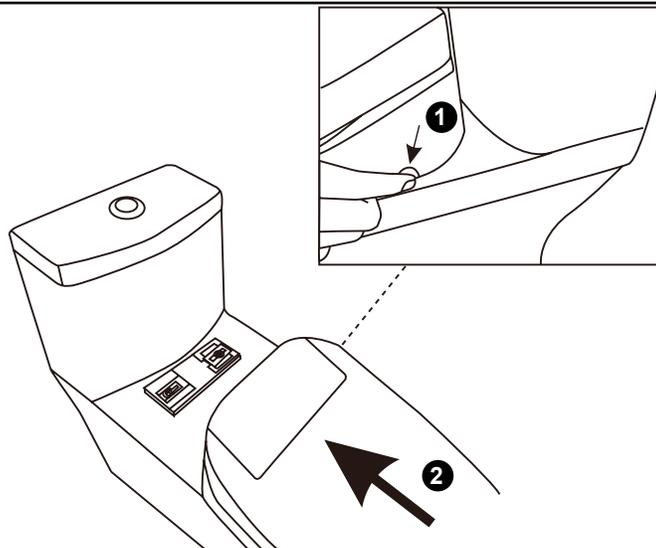
Press the release button located on the left of the seat and push the seat onto the mounting plate. Once the seat is snugly fitted onto the mounting plate, release the button and the seat will be locked in place.
