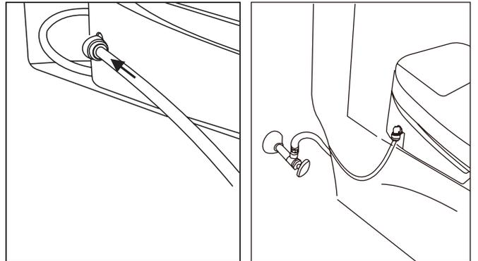
Connect the water tube to the smart seat. This is a pressure snap-in system, gently but firmly push the tube inside the hole.
