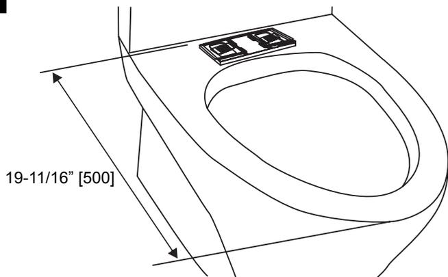
Before tightening the mounting plate, ensure that the distance between the back of plate and front edge of the toilet bowl is set to 19-11/16" (500mm). Then tightly secure the plate.
