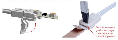
Once tape is fully inside connector, close and lock pressure pad door.
