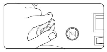
4. Pull the choke knob out to the "Choke" position.
