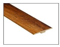
T-molding transition piece is used to transition between floors of the same height. It is usually used to provide expansion gaps for large areas or for when the floor is interrupted by wall openings or permanent fixture such as a kitchen island. The T-molding does not come with a track. It is to be installed by gluing one side of the "T" to one section of the flooring. This installation will still provide an expansion gap for the floating floor.
