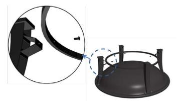
**Step3:** Attach the four legs (E) to the fire bowl (D) by M6\*10 Bolt (CC). Please DO NOT tighten the bolts at this time.
