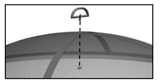
Step1: Insert Screen Handle (A) into hole in Mesh Screen (B) and tighten it with Nut (AA) underside to secure.
