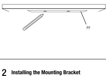
Screw in the Mounting Brackets (EE) using the Mounting Screws (DD) on the marked locations.
