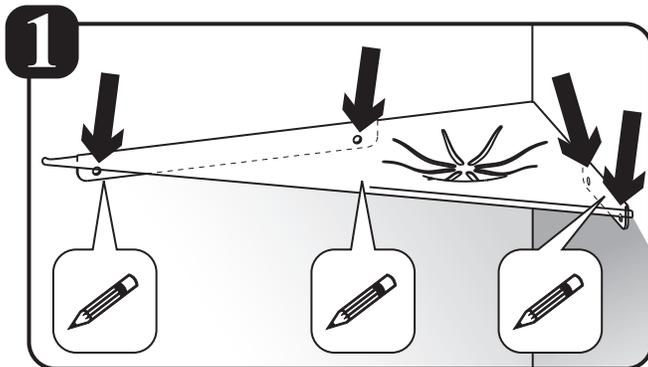
Mark positioning of the screw holes.
