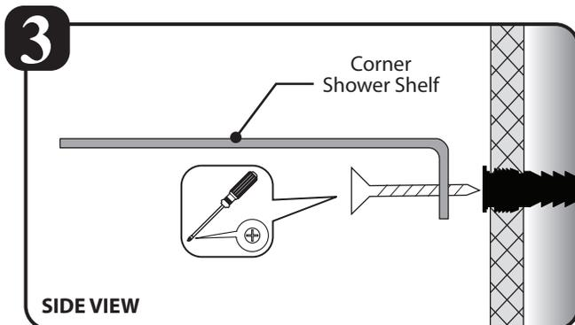
Place the shelf over the tile anchors and tighten firmly with Phillips head screwdriver.
