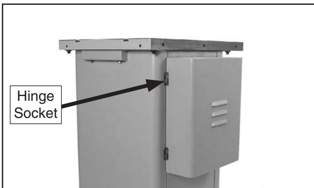
Figure 17. Motor door installed.
