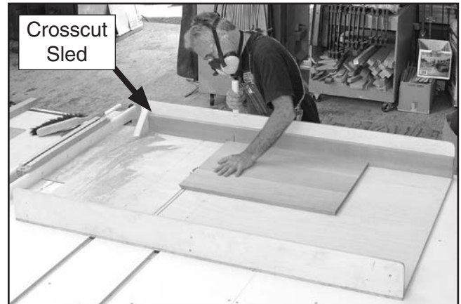
Figure 94. Example of crosscut sled.
