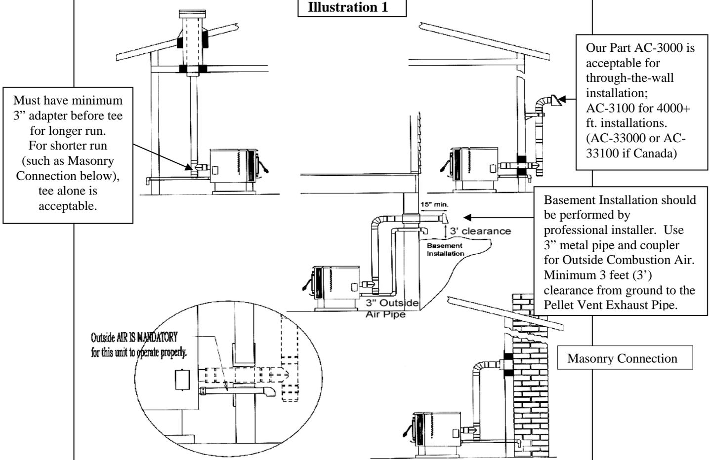
1. If 3" flue pipe exceeds 15' in length, increase to 4" flue pipe for remaining flue connections.
