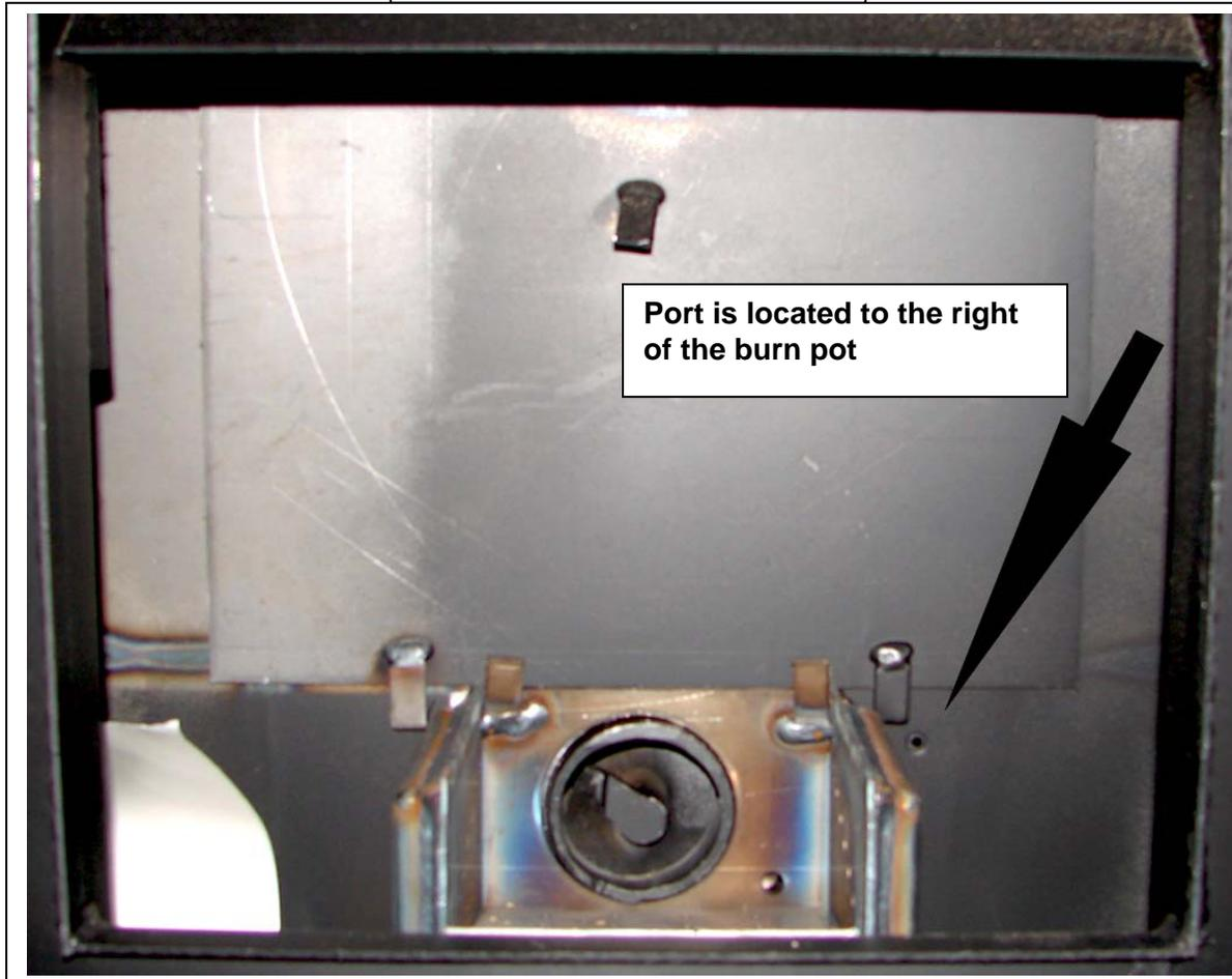
**NOTE:** The "door ajar" vacuum switch port must be kept clean, or the top auger will cease to function. Locate the port hole to the right of the burn pot and, with the stove unplugged and cooled down, use a brush or pipe cleaner (not a vacuum) to keep this port clear of ash or other debris (see picture).
