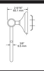
MATERIALS: Base Plate, Post and Handle Screw - Zinc Die Cast
